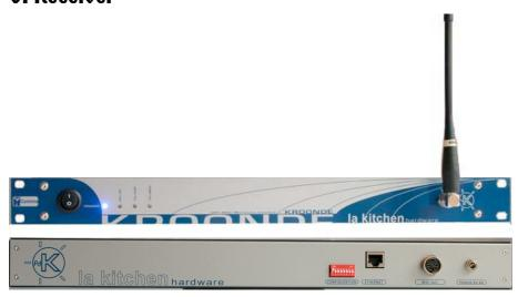
The receiver is a 1U rack, with a power switch, 4 LED's and a antenna in the front. On the rear there is a 9 V AC 500mA power supply, 1 MIDI Out connectors, a RJ45 jack for the Ethernet connection (10Mb/s) and 8 configuration microswithes.
