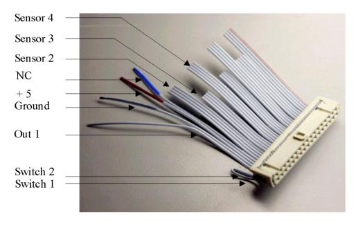
The first two wires (switch 1 and switch 2) must always be linked together. The other wires are identical, in groups of 4 for each sensor.
